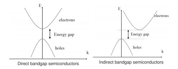
Diagram 2: This diagram shows the two different type of band gap: direct and indirect band gap with energy plotted against wave-vector. [12]
