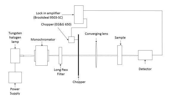
Diagram 4: Experimental set up with the apparatus mounted on a metal track.
