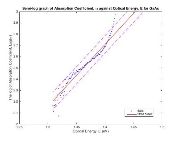
Graph 1: A semi-log graph of absorption coefficient,  $\alpha$  being plotted against the optical energy, E, in order to investigate the Urbach slope. The inverse of the gradient of the line of best fit of the band tail is the Urbach slope.
