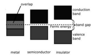
Diagram 1: This diagram shows the difference between the band gap of metal, semiconductor and insulator. [9]
