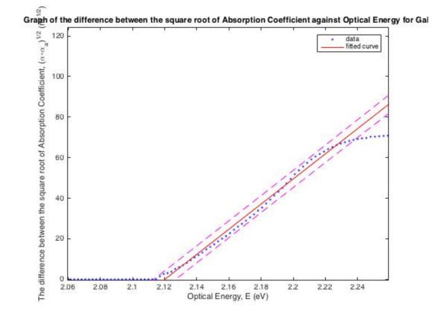
Graph 4: A graph of square root of the difference between the absorption coefficient,  $(\alpha - \alpha_a)$  against optical energy, E.The x- intercept of the line of best fit of the linear part of this graph is  $E_g + E_p$ .
