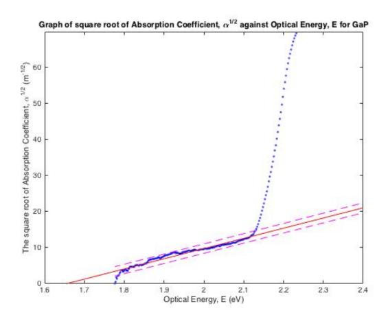
Graph 3: A graph of the square root of absorption coefficient,  $\alpha^{1/2}$ , against optical energy, E, for GaP. The x- intercept of the line of best fit of the linear part of this graph is  $E_g - E_p$ .
