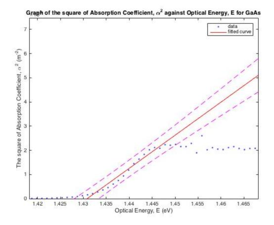
Graph 2: A graph of the square of absorption coefficient  $\alpha^2$  being plotted against the optical energy, E, in order to investigate the band gap energy of GaAs. The xintercept of the line of best fit of the linear part of this graph is the band gap energy.
