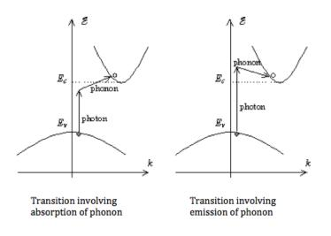
Diagram 3: This diagram shows the two different ways electrons can transition from the valence to the conduction band in an indirect band gap semiconductor. [17]
