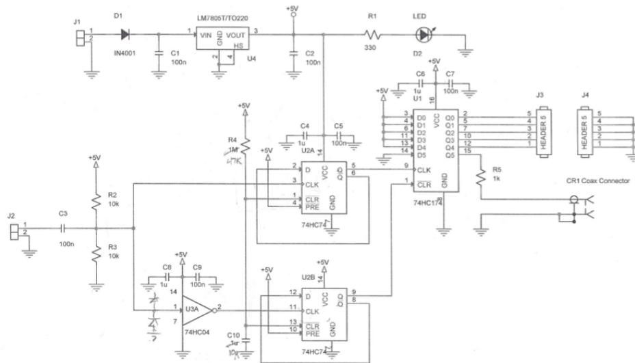
Figure 3: Ground bounce circuit schematic.
